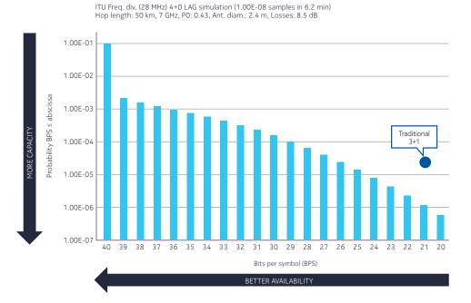
Figure 2. Multichannel versus traditional N+1 scaling and protection
