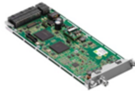
PLUGIN CARDS – ETHERNET WITH 1 COMBO AND 3 ELECTRICAL OR OPTICAL INTERFACES
