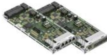
PLUGIN CARDS – ETHERNET WITH 1 COMBO AND 3 ELECTRICAL OR OPTICAL INTERFACES
