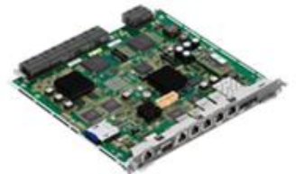
PLUGIN CARDS – ETHERNET WITH A SINGLE 10GE OPTICAL INTERFACE
