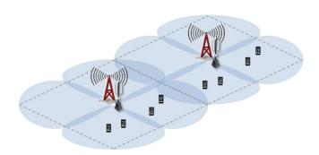
Co-locate A8n (ac) with existing 3G/LTE cell site to offload traffic for an almost identical cell area.
